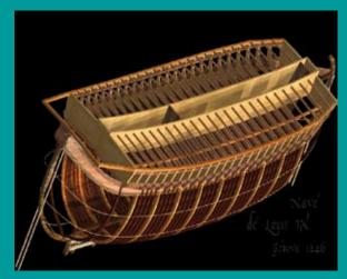
The modell shows a detail of Acre Harbour from the middle of the 13th century earlier than 1291. Two scientifically researched and historically documented types of ships are shown true to detail: A galley, called Tarida, which was built for the the armada of Karl of Anjon in 1274 equipped for 108 oarsmen. Moreover there is a nave from 1246, a ship for 450 pilgrims, from the armada of Ludwig IX, who was known as the Saint.
